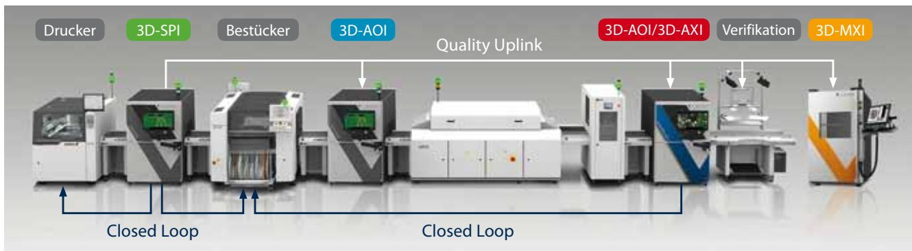
Inspection-line in SMT production
